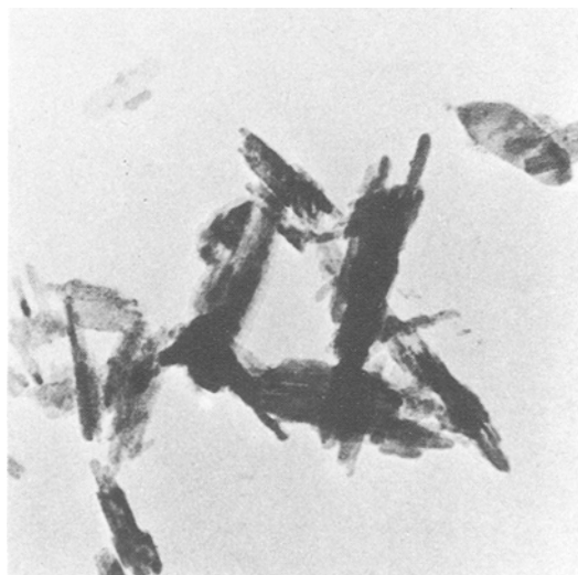
Figure 2 Transmission electron microscopy of original synthetic lepidocrocite powder (magnification \times 35\,000 ).
